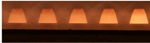
**Figure 3.9:** Cross-section of an array of ablated waveguides in Truemode, the waveguides have a cross-section of  $\approx 50\mu\text{m} \times 50\mu\text{m}$  on pitch  $125\mu\text{m}$ . The waveguide core has a height of  $50\mu\text{m}$  and a width of  $45\mu\text{m}$  at the top of the core layer and  $60\mu\text{m}$  at the bottom of the core layer.
