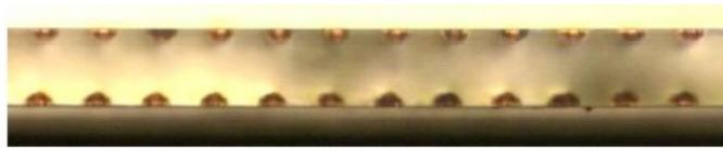
**Figure 1.6:** Double-sided optically functionalized thin glass with waveguide dimensions of approx.  $53 \mu\text{m} \times 110 \mu\text{m}$ , fabricated by silver-ion exchange using a salt melt [15].
