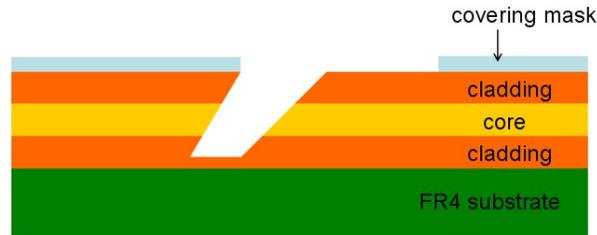
**Figure 4.27:** Schematic showing the alignment of the tape with respect to the ablated trench. The sidewall of the opening in the mask is aligned with the polymer-air interface of the ablated mirror in order to avoid the deposition of Au onto that interface.
