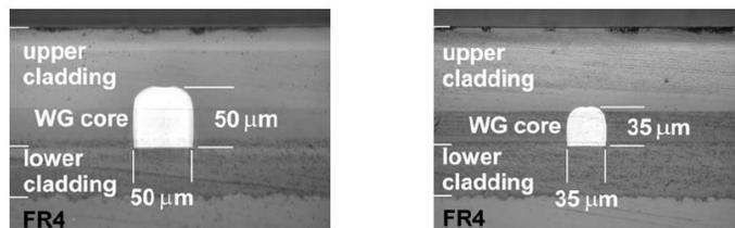
**Figure 1.7:** Cross-section of a polymer waveguides with a cross-section of  $50 \mu\text{m} \times 50 \mu\text{m}$  (left) and  $35 \mu\text{m} \times 35 \mu\text{m}$  (right) [18].
