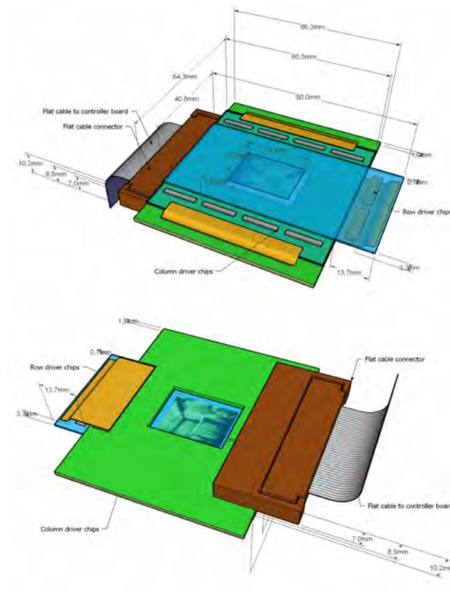
Figure 3.36: The designed end result for the HeMind module
