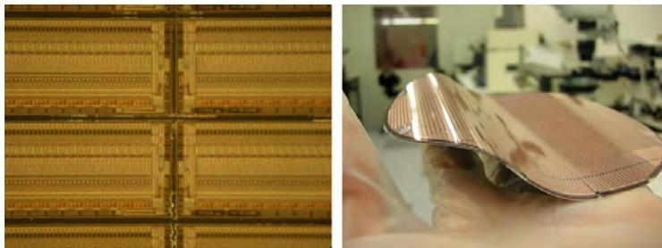
Figure 6.36: A diced wafer (with the sawing lanes visible left) gives a false impression of flexibility (right)
