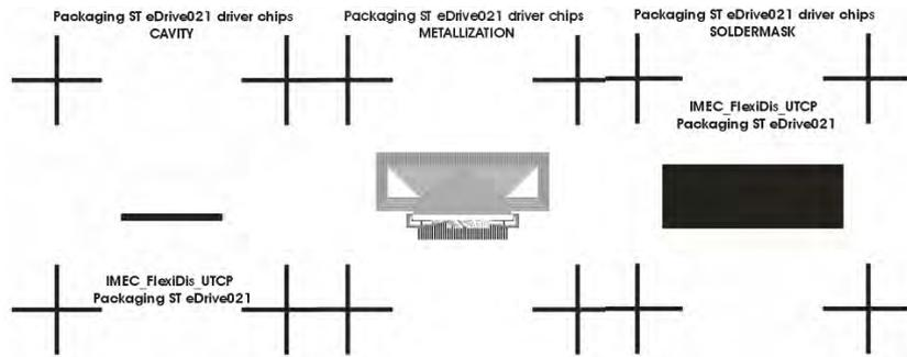
Figure 6.41: Designed masks for the UTCP to match the eDrive021 chip
