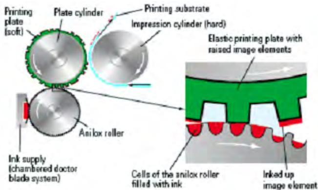
Figure 2.26: Principle of flexography
