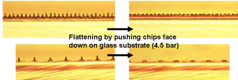
Figure 3.48: Flattening the studbumps to lower locally induced pressure during bonding
