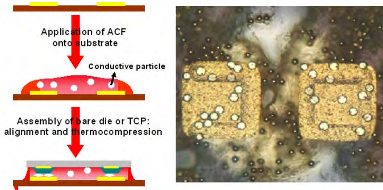
Figure 2.41: Principle of assembly technology using ACF
