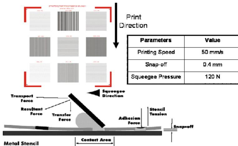
Figure 2.14: Stencilprinting setup: print direction and parameters
