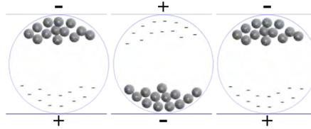
Figure 1.8: Principle of an electrophoretic display
