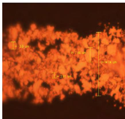
Figure 2.16: Stencilprinting results: zoomed top view of the smallest printed lines
