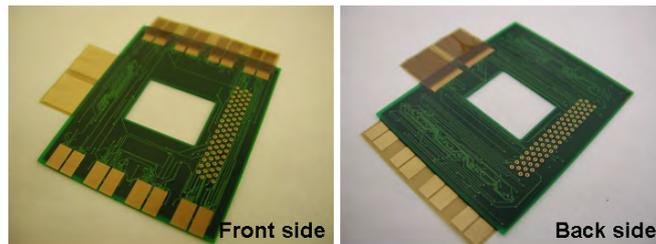
Figure 3.35: The underlying PCB for rerouting all driver input signals from a cable connector to the appropriate drivers
