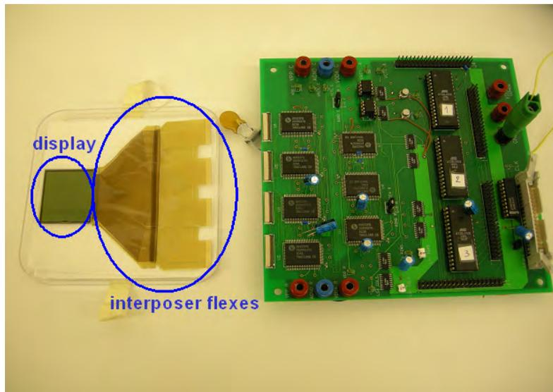
*Figure 3.1: Interconnecting a display using an interposer flex: the display is intended for a cellphone, the PCB (on the right) is used for testing drive schemes (obviously far too big for an actual cellphone, see also Figure 2.4)*
