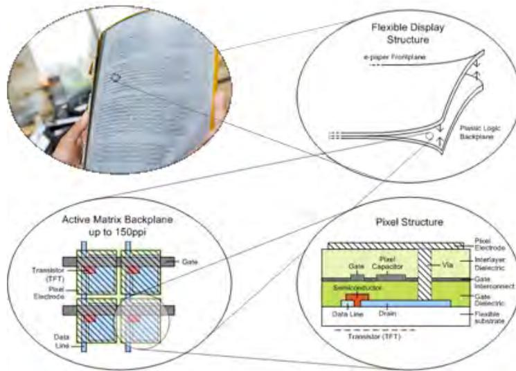
Figure 4.3: Plastic Logic's flexible backplane is combined with a frontplane material (e.g. electronic paper) to make a flexible display (from their website)
