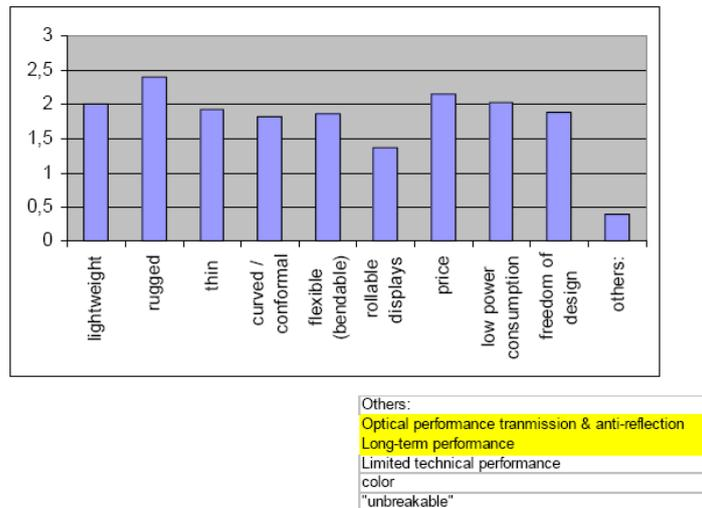
Figure 5.10: A questionnaire illustrates which properties might be important for flexible displays as considered by european flexible display consortium (FlexiDis) members
