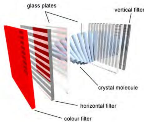
*Figure 1.6: Working principle of liquid crystal technology*
