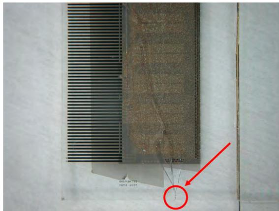
Figure 3.46: The crack in the glass originates from the glass edge
