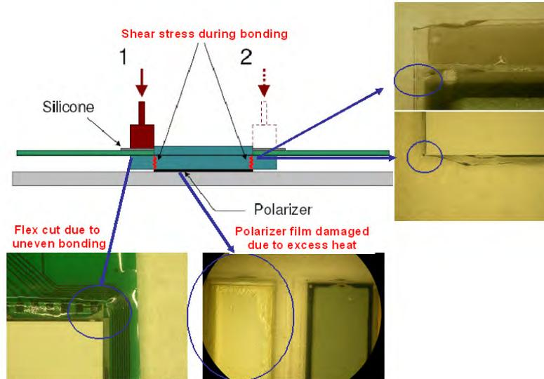
Figure 3.16: Issues with the initial bonding setup
