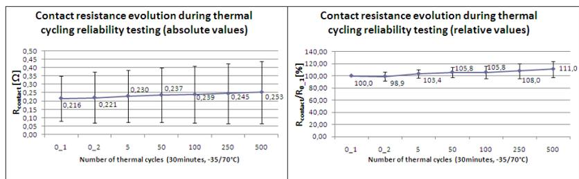
Figure 6.47: Thermal cycling reliability in absolute and relative values
