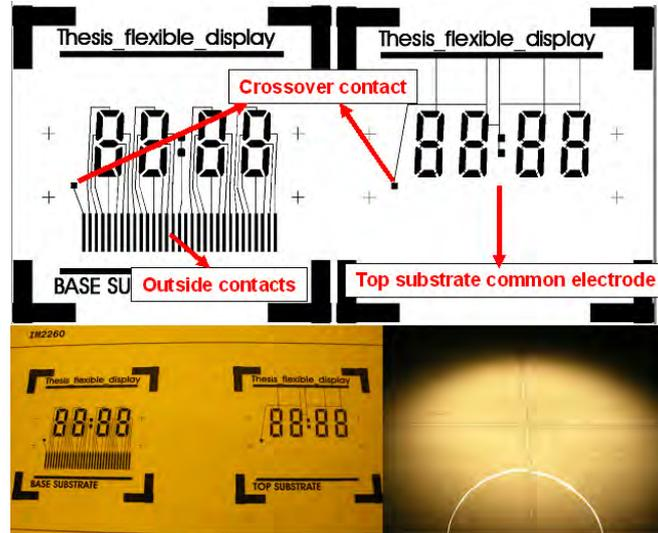
Figure 4.33: Design of the final PDLC display demonstrator (top), as well as the corresponding mask set (on foil, below left) and some patterned substrates (difficult-to-see transparent ITO patterns on PES substrates, still attached to the carrier, below right)
