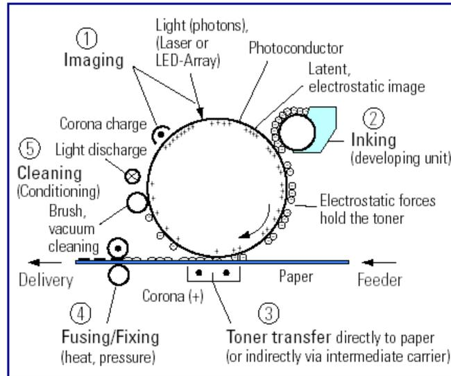
Figure 2.30: Laserprinting principle
