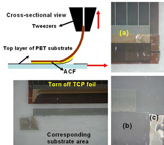
Figure 4.24: Results for peel strength tests along the bond length: the top layer of the PET substrate is torn loose and remains attached to the TCP foil (a), a void area is left behind on the PET substrate (b), with the exception of some adhesive leftovers at the sides (c)
