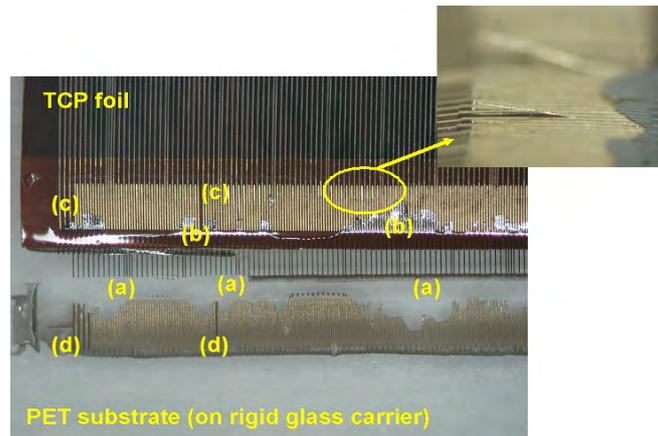
Figure 4.23: Resulting surfaces after peel strength testing perpendicular to the bond length: in some areas a layer (with gold metallization) is torn from the PET substrate (a), and still clings to the TCP foil (b), in other areas, copper traces are torn from the TCP foil (c) and still cling to the substrate (d); the zoomed view shows a copper trace that is partially torn off the TCP foil, while at the same time a layer of the PET substrate is still sticking to the TCP foil
