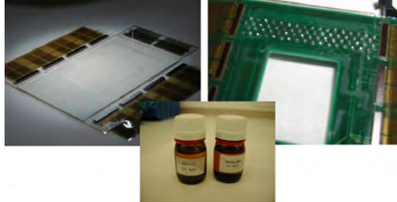
*Figure 3.43: The status of the display assembly before (left) and after (right) gluing the display to the PCB; the 2-component epoxy adhesive is shown in the middle*
