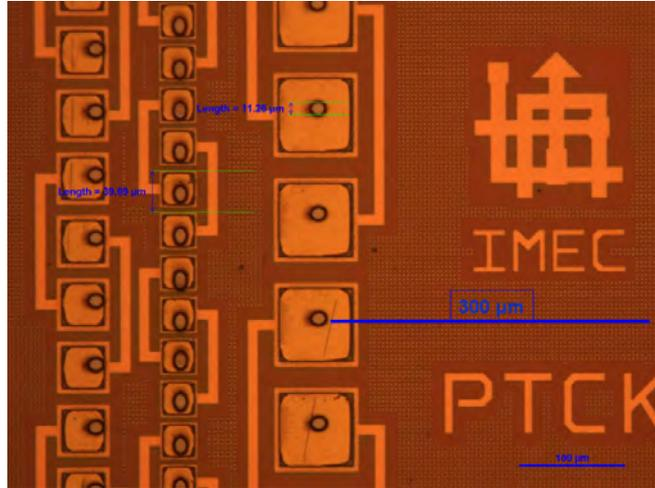
Figure 6.10: Laser drilled via holes in the top PI layer to contact the bumped contact pads of the chip underneath, for all three types of bond pads
