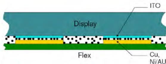
Figure 3.15: Principle of ACF for bonding the watch displays
