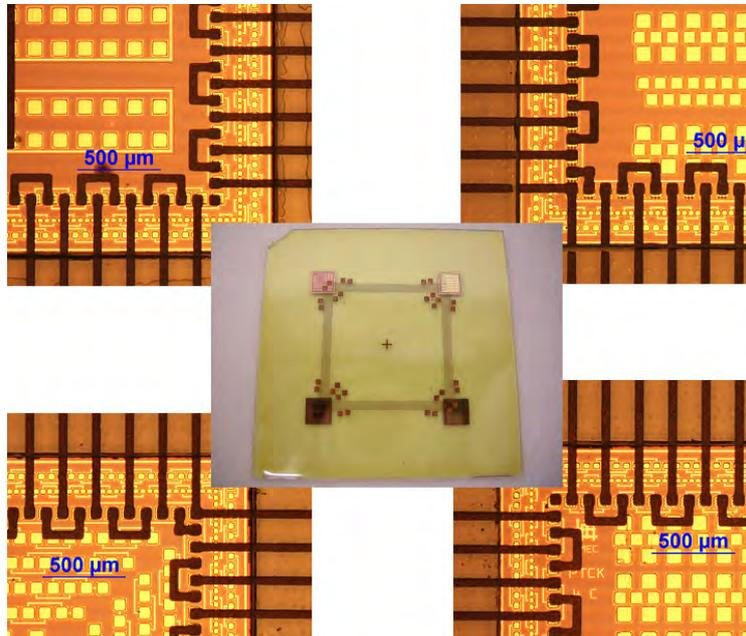
Figure 6.45: Alignment of the chips at the four corners to the metallization is sufficient for interconnection
