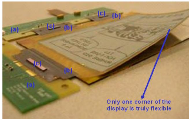
Figure 5.1: Flexibility issues in flexible display modules: (a) external driving electronics on rigid PCB, (b) TCP attachment and (c) rigid Si driverchips
