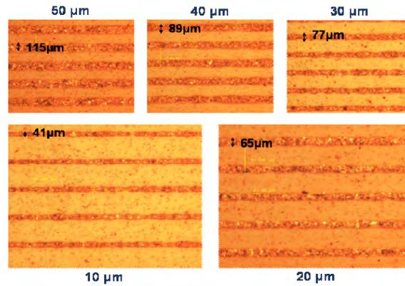
Figure 2.15: Stencilprinting results, clockwise from the top left corner: results from the 50, 40, 30, 20 and 10 micron stencil openings (all are 250  $\mu\text{m}$  pitch)
