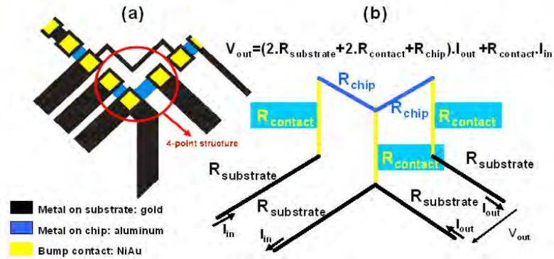
Figure 4.5: Principle of 4-point measurement: (a) top view and (b) “3D”-view explaining the principle
