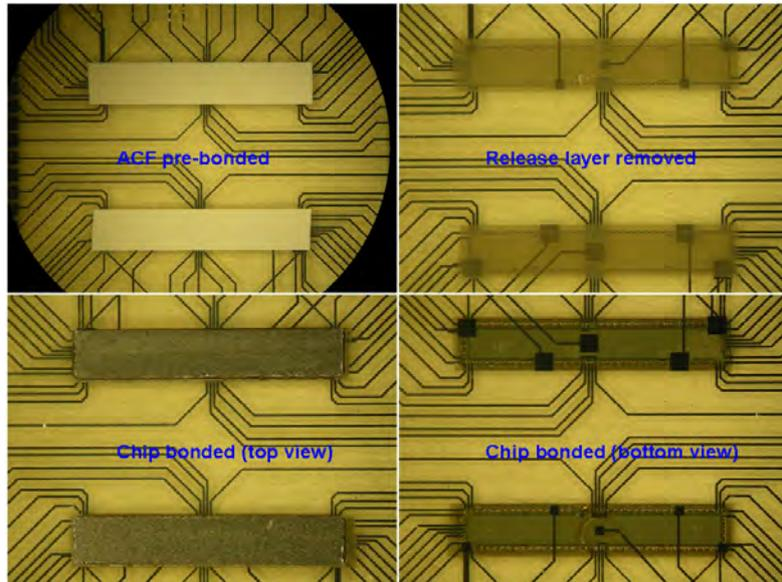
Figure 3.25: The sensor matrix bonding process in pictures: the small and large square photodiodes are visible underneath the chip (under the middle of the chip as well as underneath the peripheral bond pads themselves)
