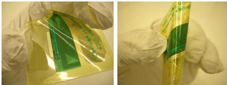
Figure 6.42: First UTCP trials with functional driver chips embedded
