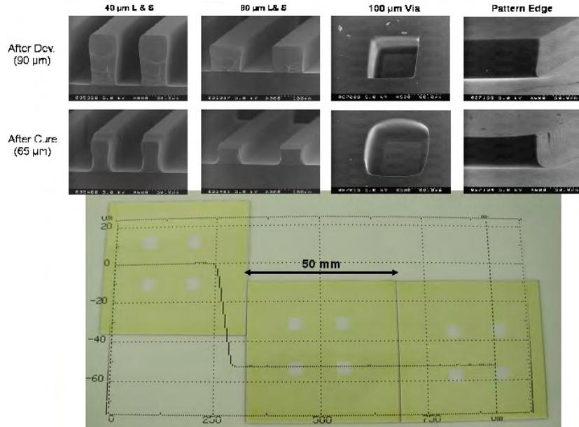
Figure 6.6: Defining cavities with the photodefined HD7012: SEM pictures from results in the datasheet (top) and cavities achieved (bottom)
