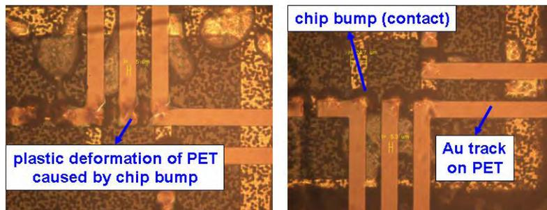
Figure 4.14: Pictures of a flip chip assembled 50- $\mu\text{m}$ -pitch test chip: the contacts are pressed slightly into the substrate
