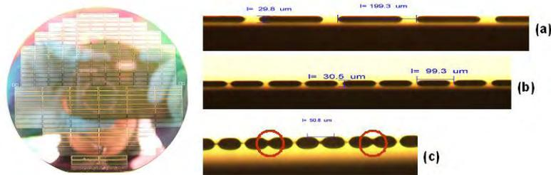
Figure 4.7: Resulting chips of the 1<sup>st</sup> batch: pitches (a) 200  $\mu\text{m}$ , (b) 100  $\mu\text{m}$  and (c) 50  $\mu\text{m}$  (overplated and shorted)
