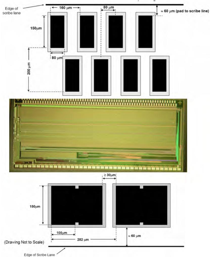
Figure 3.21: The read-out chip ISC9717: input pads (top) are staggered  $160\mu\text{m}$  by  $80\mu\text{m}$  pads at a pitch of  $160\mu\text{m}$ , while the output pads (bottom) have the approximately the same size ( $150\mu\text{m}$  by  $100\mu\text{m}$ ) but have been paired up at a pitch of  $282\mu\text{m}$
