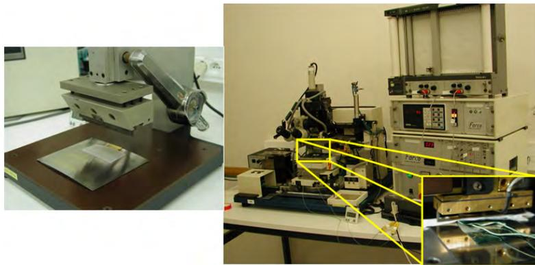
*Figure 2.43: Bond equipment: the manual heat seal machine (left) and the semi-automatic bonder (right, setup with thermocouples for trials checking the temperature profile at the bond area)*
