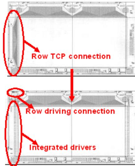
*Figure 5.6: Integrating the row drivers in the backplane design greatly reduces the number of interconnections, while the space on the backplane taken away from the active area is practically negligible*
