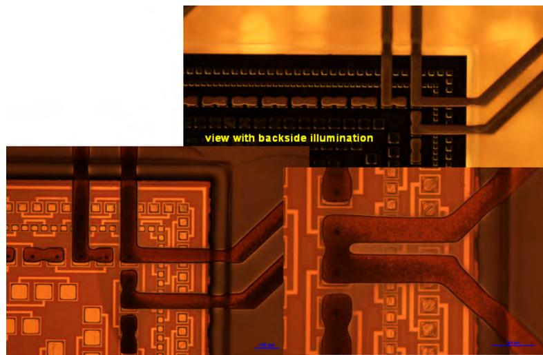
Figure 6.32: Good results with adequate gap crossings at a coarser pitch of  $100\ \mu\text{m}$
