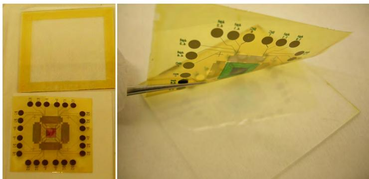
Figure 6.26: Optimized UTCP release: formerly by cutting out the middle part (adhesion promotor applied at the sides of the glass carrier, left picture), currently the glass can be reused after release of the UTCP (right picture)
