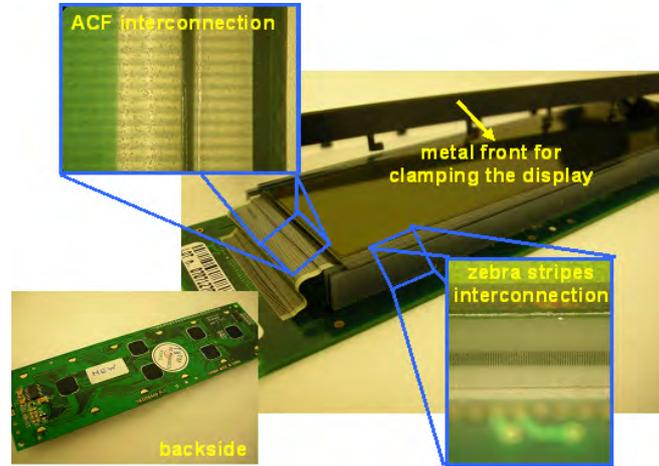
Figure 3.6: A display with ACF interconnection for the rows and zebra stripes for the columns: the electronic circuitry is assembled on the backside of the PCB, and the zebra stripes are clamped between display glass and PCB by a metal front
