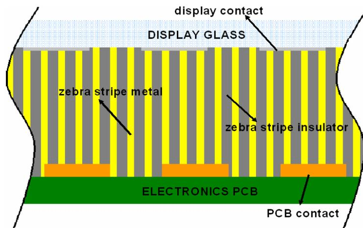
Figure 3.4: The principle of a zebra stripes interconnection
