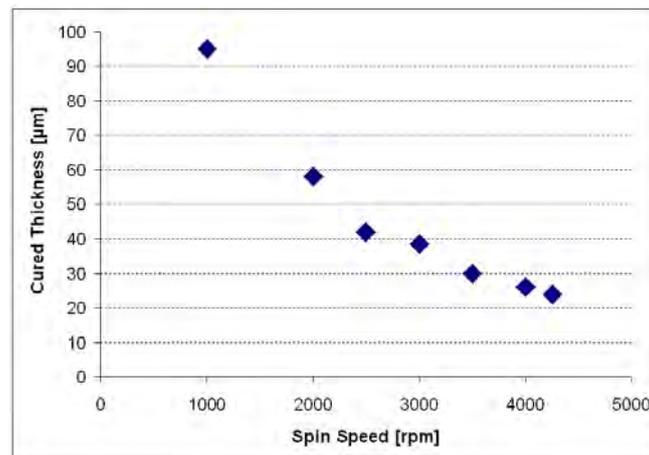
Figure 6.27: Spin speed curve for HD7012: useful for matching chip thickness and cavity depth
