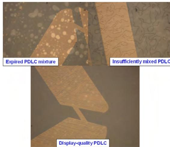
Figure 4.39: Problems encountered with the PDLC mixture
