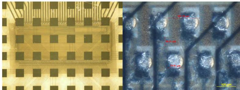
Figure 3.30: Results of the assembled demonstrators: an ACF bonded chip (left) and a close-up of the input area of the read-out chip (right, the studbumps are aligned to the contact pads on the substrate)
