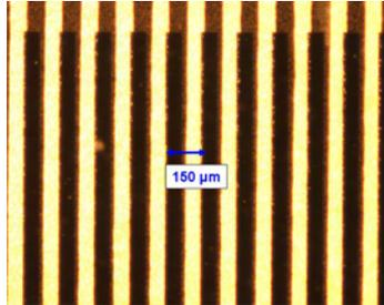
Figure 4.21: Despite misalignment electrical interconnection is still ensured through the ACF particles (indents still visible in the tiny overlap areas)
