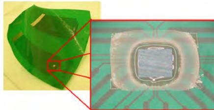
Figure 4.1: Chips assembled on a PI substrate
