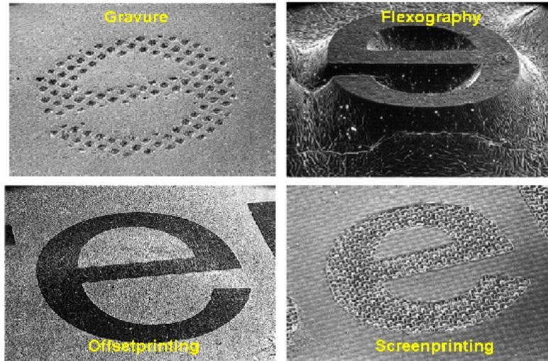
Figure 2.28: Masterplates for the various printing technologies (except for inkjet obviously): note that master plates for gravure and flexography require mirrored patterns
