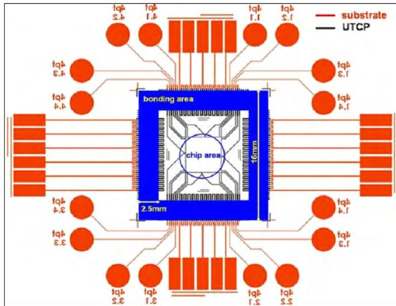
Figure 6.16: General layout of the UTCP assembly design
