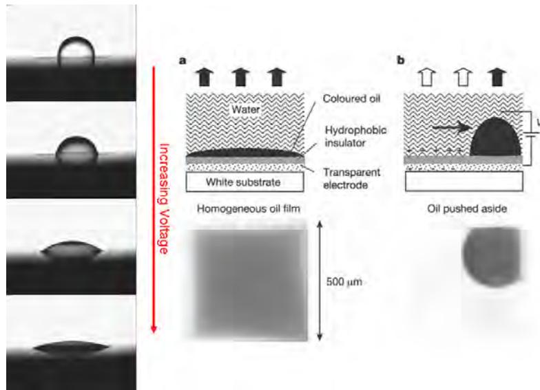
Figure 1.13: The principle of electrowetting illustrated (Liquavista): no voltage applied, therefore a coloured homogeneous oil film is present (a), DC voltage applied, causing the oil film to contract (b)
