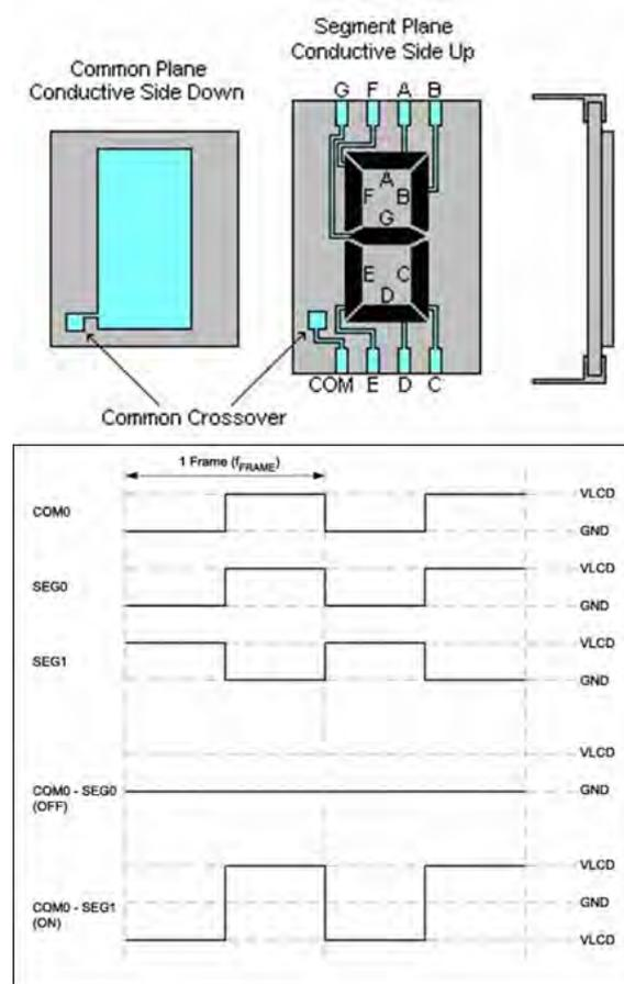
Figure 1.22: Implementation and waveforms for a static LCD
