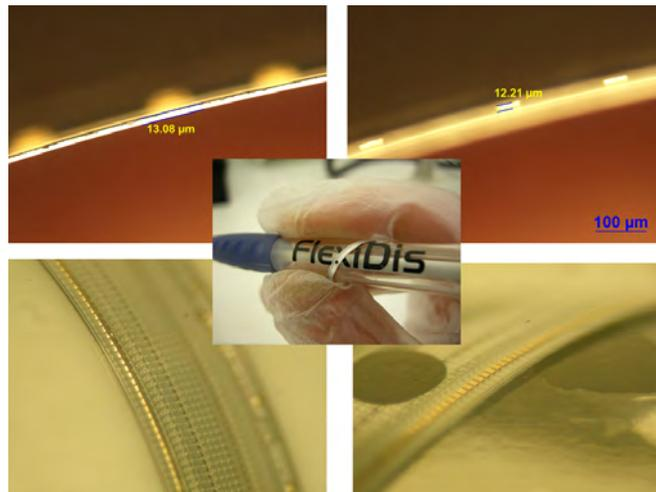
Figure 6.40: Some more results of the fly-cutting and thinning process: chip thinned down to 13  $\mu\text{m}$ , chip bumps are 12  $\mu\text{m}$
