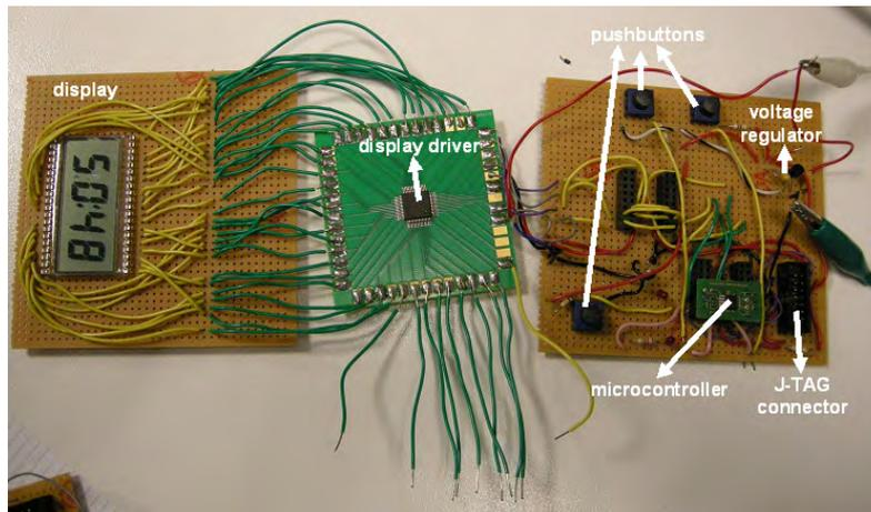
*Figure 4.43: A testing prototype for the driving electronics: the standard LCD display is driven with the higher voltages needed for the PDLC display*
