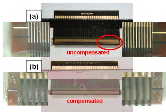
Figure 4.18: (a) Expansion leads to mismatch at the edges after bonding. (b) Compensation of expansion minimizes mismatch.
