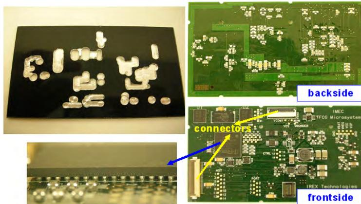
Figure 5.3: Double-sided assembly of a flexible PCB for the driving electronics: insets are created in the carrier fitting the components, namely the smaller passives, on the backside; the larger packages, including a very large IREX BGA, are assembled at the frontside
