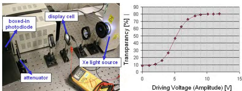
Figure 4.40: The setup for initial characterization: the photodiode is boxed-in to shield it from ambient light (preferably the measurement is carried out when the room is obscured), the incoming light spot is controlled in size by the diaphragm in front of the light source, and the attenuator (4 25-nm TiW sputtered glass substrates) is required because the used avalanche photodetector is very sensitive and would otherwise be saturated
