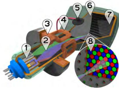
Figure 1.4: Principle of a color CRT: (1) Electron guns (2) Electron beams (3) Focusing coils (4) Deflection coils (5) Anode connection (6) Mask for separating beams for red, green, and blue part of displayed image (7) Phosphor layer with red, green, and blue zones (8) Close-up of the phosphor-coated inner side of the screen
