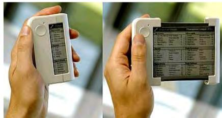
Figure 5.9: The RADIUS (PolymerVision) is a nice example of how the flexibility (rollability) of the display is optimally used, while the electronics and interconnection area is reinforced and protected by the rigid casing
