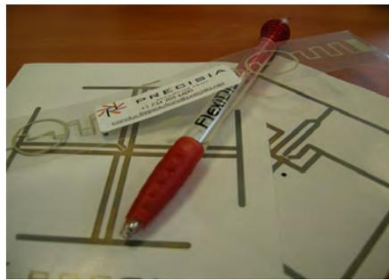
*Figure 2.23: Achievements of Precisia with regards to printing Ag ink RFID patterns on flexible paper and PET substrates*
