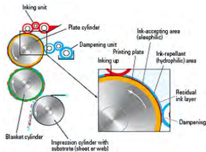
Figure 2.27: Principle of offsetprinting
