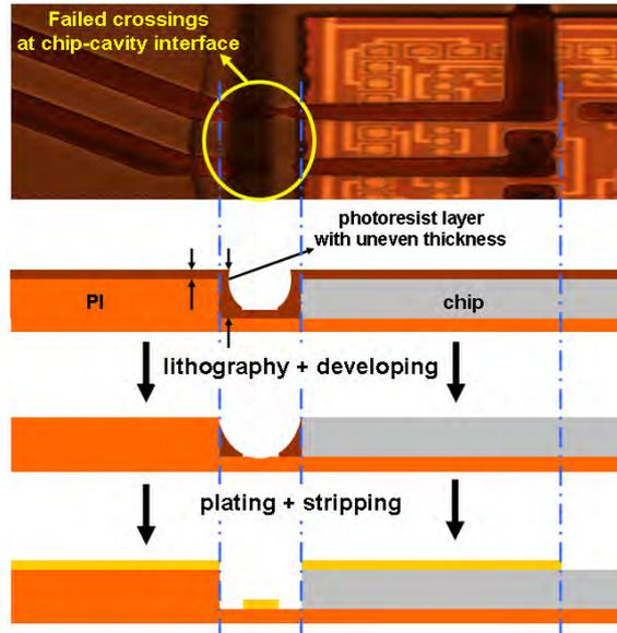
Figure 6.29: Bridging the gap at the chip-cavity interface is a challenge that needs to be addressed
