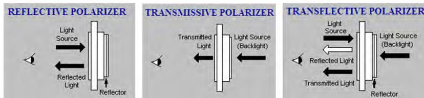
Figure 1.19: Light transmission modes for LCDs
