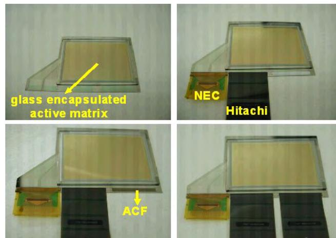
Figure 4.30: Assembly of a flexible display on a stainless steel substrate with row (NEC) and column (Hitachi) drivers packaged as TCP
