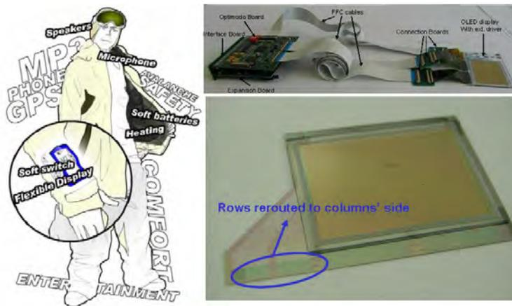
Figure 5.5: Concept (Pulsium) of a flexible display in a ski jacket's sleeve, as demonstrated within FlexiDis: rerouting the row contacts to the column side allows one-dimensional bending (electronics by Thomson)
