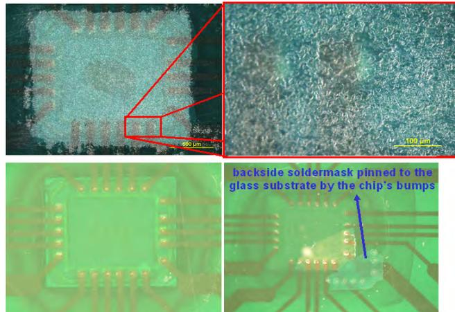
Figure 4.2: Illustrating the influence of different carrying substrates used during thermocompression: bonding carried out on a ceramic (top) and on a glass (bottom) carrier
