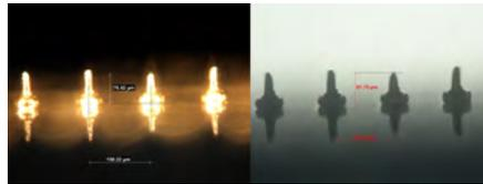
Figure 2.44: Side view of Au studdumps on a Si chip, with top (left) and bottom illumination (right)
