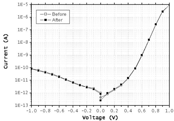
Figure 3.27: Current-Voltage characteristic in dark conditions of a photodiode before and after the flip-chip process
