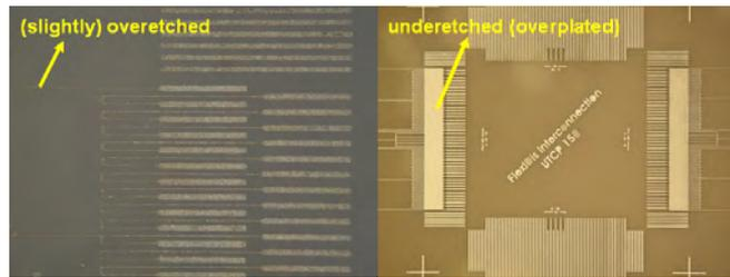
Figure 6.18: Issues etching the thin staggered output patterns on the PI substrates: either overetching (left) or underetching (right) was observed
