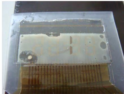
*Figure 4.46: Embedding the display in silicone could be used for protecting it from degrading influences such as moisture and increasing its mechanical ruggedness, e.g. by applying a thicker silicone layer in the display area, redirecting all stresses towards the thinner silicone areas outside the display area*
