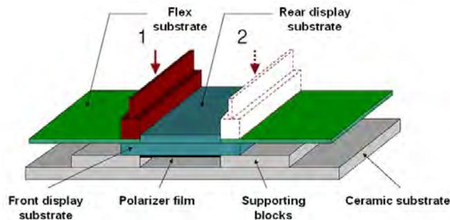
Figure 3.17: Adapted setup for bonding the watch displays: schematic
