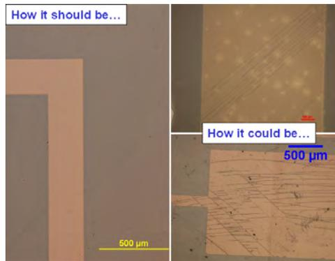
Figure 4.35: ITO is a very brittle material: cracks are easily introduced during release of the substrates (pictures on the right)
