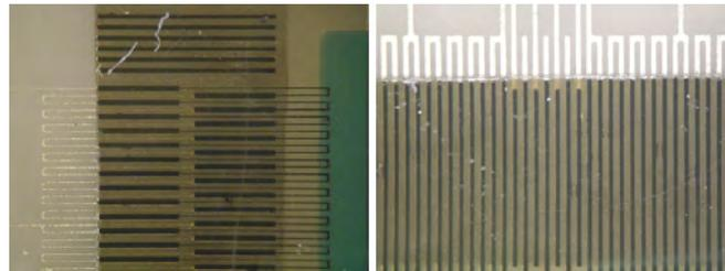
Figure 6.19: Assembly close-up with successful alignment for the smallest pitches
