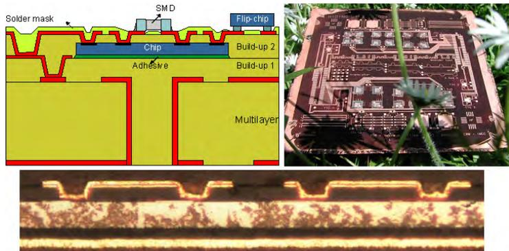
Figure 5.14: Research within “Hiding Dies” involves embedding thin dies in the buildup layers of a PCB
