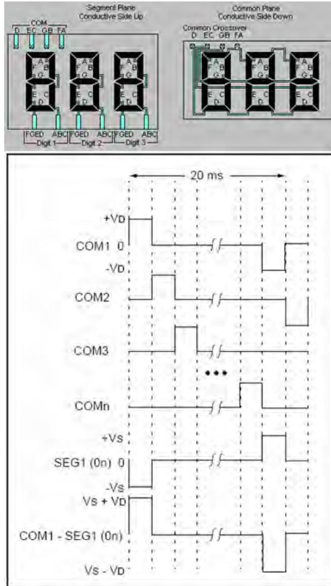
Figure 1.23: Implementation and waveforms for a multiplexed LCD
