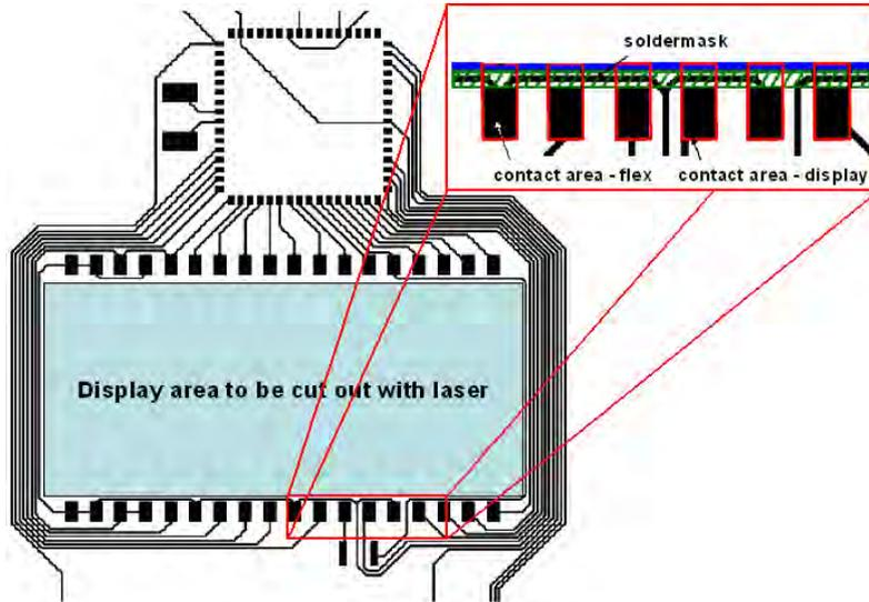
Figure 3.14: Routing pattern for interconnecting microcontroller and display on a single-sided flex substrate
