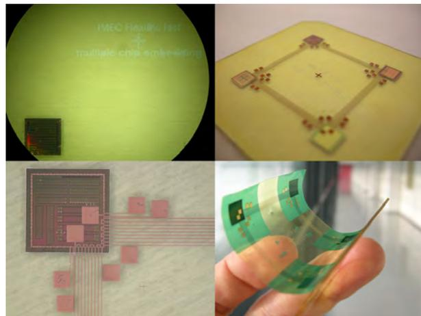
Figure 6.44: Several pictures of the fabricated substrates with embedded chips: a placed chip (top left), 4 embedded chips interconnected by the Cu metallization layer (top right), a close-up (bottom left) and the end result, with soldermask and NiAu finish (bottom right)
