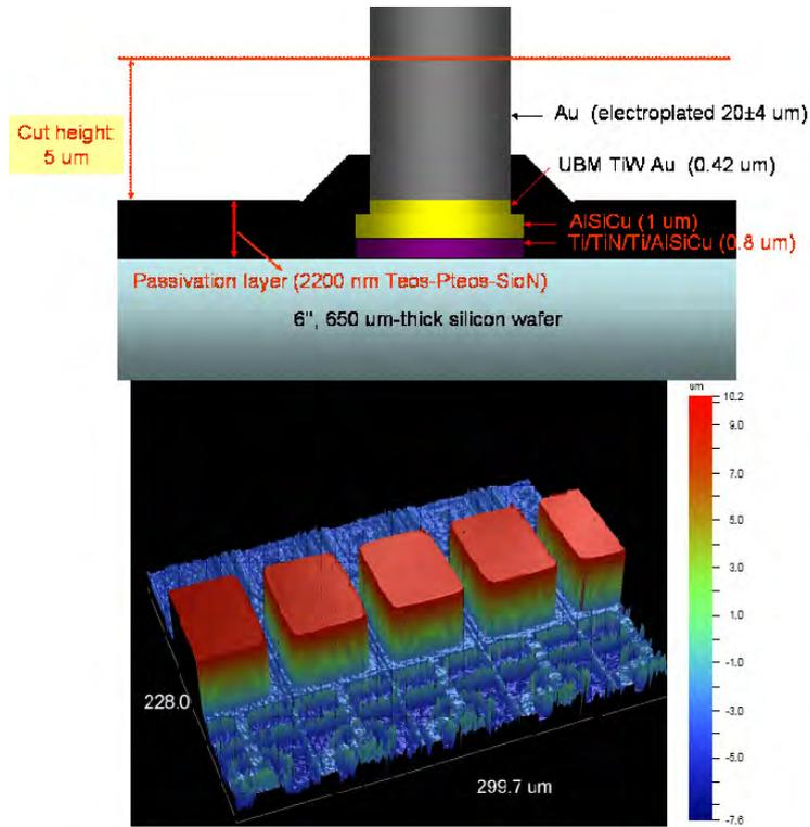
Figure 6.35: Specifications and results of flycutting the STM wafers: instead of the asked 5  $\mu\text{m}$ , the bumps were fly-cut to approximately 12  $\mu\text{m}$
