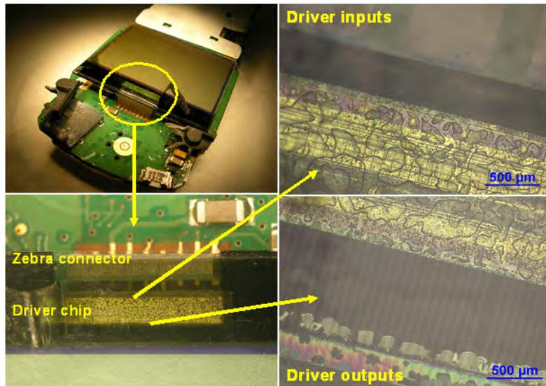
Figure 3.3: Disassembly of a cellphone: the driver chip is directly mounted on the glass of the LCD, and the (fewer) inputs are connected to the electronic circuitry by zebra stripes
