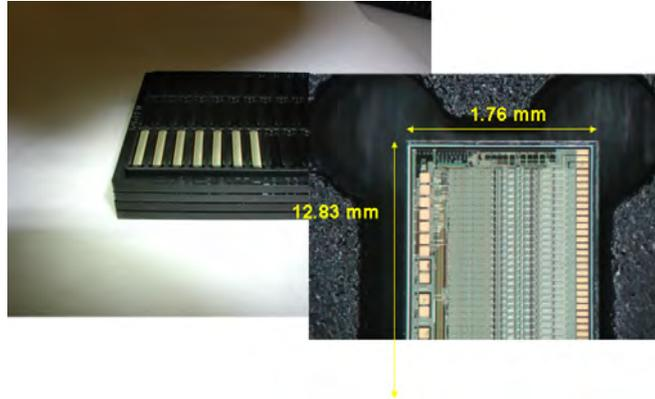
Figure 3.32: The column drivers used for the HeMind display
