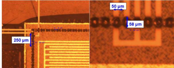
Figure 4.11: Pictures of a flip chip assembled test chip, proving the feasibility of aligning 50- $\mu\text{m}$ -pitch chips to a patterned substrate; note the overplated contacts
