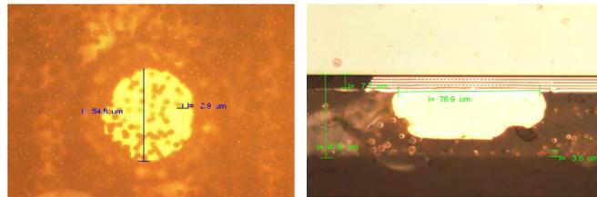
Figure 3.49: Through-the-glass-substrate view (left) and cross-sectional view (right) of an unconnected flattened bump
