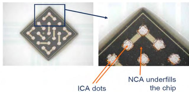
Figure 2.40: An example of adhesive assembly with isotropic conductive adhesives
