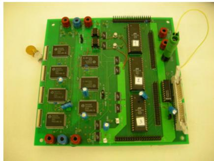
Figure 2.4: A PCB assembly for research on display driving schemes (TFMG Microsystems)
