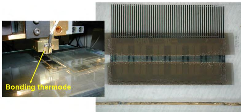
Figure 3.40: Row driver chips (being) bonded to the display
