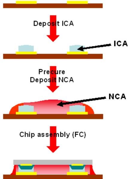
Figure 2.39: The principle of the lab's patented adhesive assembly with isotropic conductive adhesives
