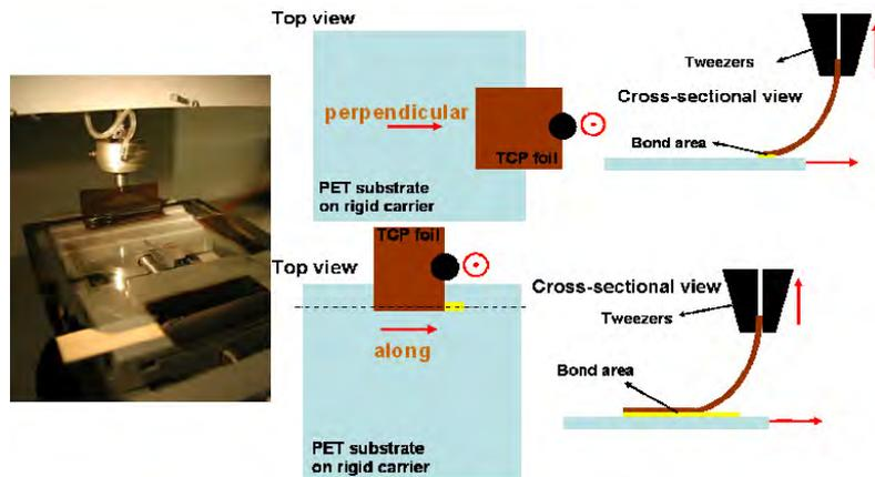
Figure 4.22: Setup for peel strength tests perpendicular (above) and along (below) the bond length; the movement of substrate and tweezer (pulling) is indicated by the red arrows
