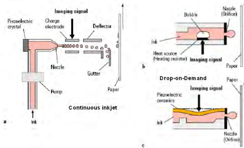
Figure 2.20: Inkjetprinting methods: continuous (a) and drop-on-demand thermal (b) and piezo (c) inkjet
