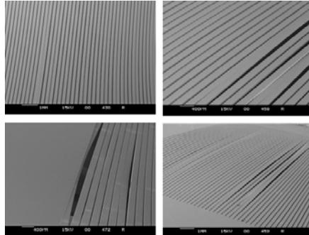
Figure 2.10: Result of stencil fabrication: the stability of the long narrow lines may lead to problems during framing and printing
