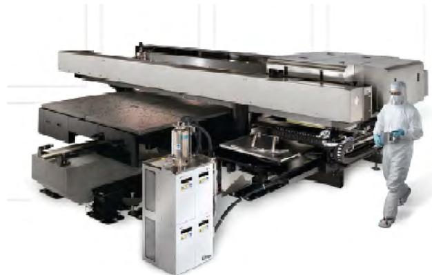
*Figure 2.22: The Litrex M-series: large area electronics inkjet printers with performance proven up to Gen 8 substrates (up to 2400mm x 2400mm), a print speed of 1000 mm/s and a drop placement accuracy of 15  $\mu$ m*
