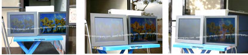
*Figure 1.20: Viewability issues on LCDs: outdoor conditions and wide viewing angles pose problems for standard LCDs (left-sided displays), but can be passively and/or actively enhanced (right-sided displays)*
