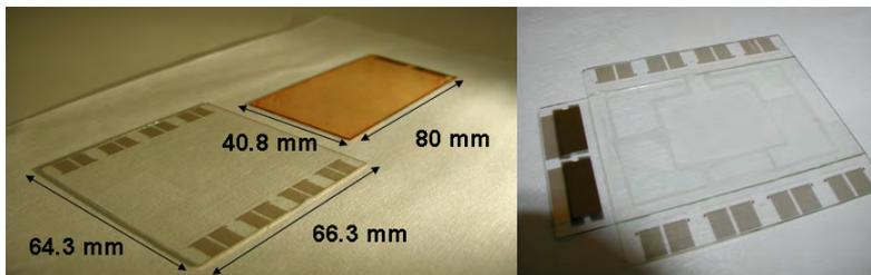
*Figure 3.31: Glass substrates for display fabrication: a column substrate on the left and a row substrate on the right (left picture) are used to fabricate a HeMind display (right picture); the row substrate in the left picture is still coated with photoresist for protection during polishing, explained in Section 3.4.3; the display active area is visible at the center of the assembly in the right picture*
