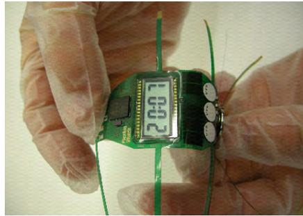
*Figure 3.8: An assembled flex watch*
