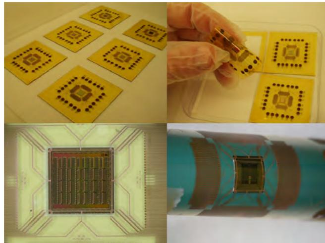
Figure 6.13: The results after the seed layer etch
