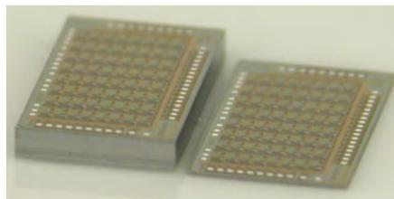
Figure 6.4: A functional chip before and after thinning
