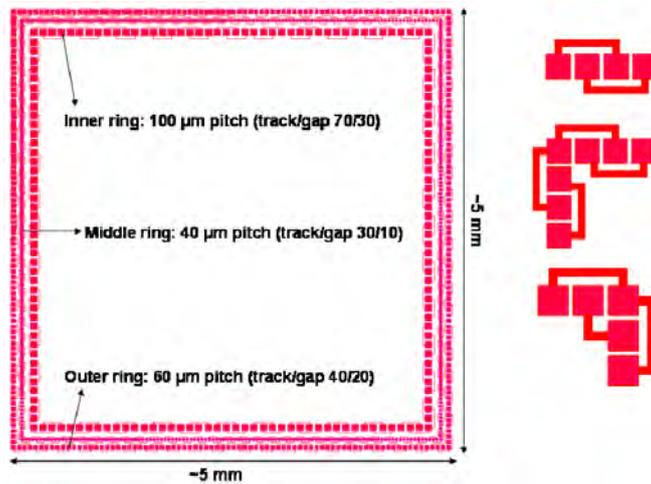
Figure 6.2: The bond pads of the PTCK test chips are located at the periphery and come in 3 pitches, 100, 60 and 40  $\mu\text{m}$ , a more zoomed view on the right shows the different interconnection schemes on the chip
