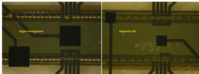
Figure 3.26: Some close-up results of the bonding trials: note the slight misalignment on the left, and the indentations on the contact pads (these are marks caused by the ACF's metal particles being pressed into the thin contact pads on the substrate during thermo-compression)
