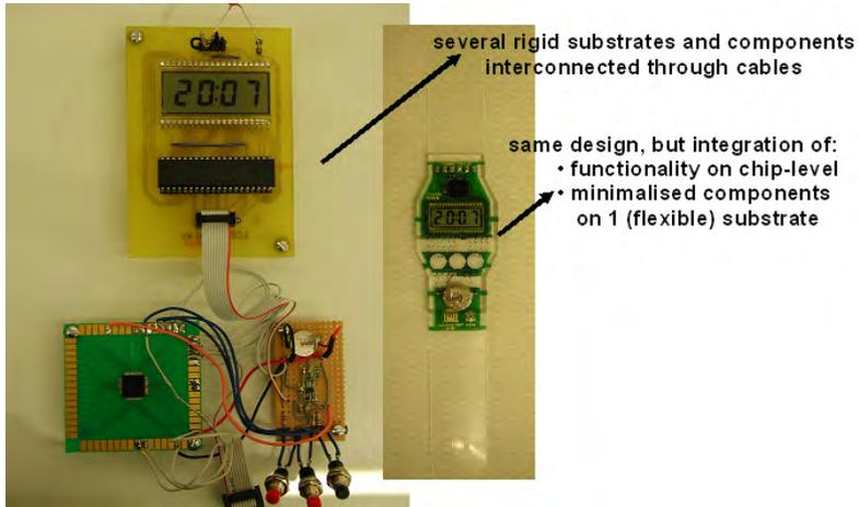
Figure 3.12: Illustration of how the choice of interconnection technologies defines size and weight of electronics: the two pictures are identically scaled
