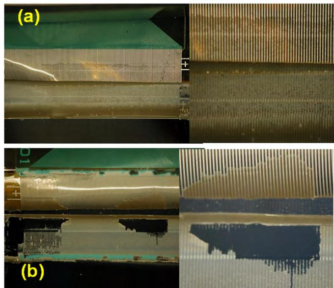
Figure 4.29: Peel strength tests on a bonded NEC TCP: (a) result of peeling along the bond length, (b) result of peeling perpendicular to the bond length
