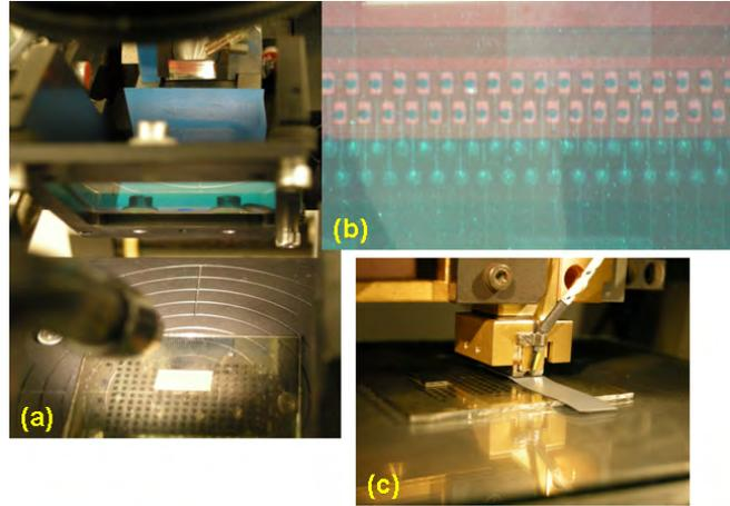
Figure 3.29: Illustrations of the assembly process: (a) the aligning and placing setup (beam-splitter in the middle, chip at the top, picked up by the chuck and substrate at the bottom of the picture) (b) a view through the aligner microscope (the round contours are the studbumps) (c) the thermocompression step (on the left one chip is already assembled, on the right the silicone interlayer covers the chip during thermocompression)
