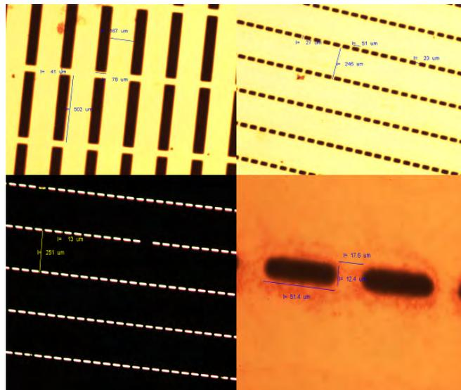
Figure 2.11: Result of stencil fabrication: clockwise from the upper left corner is shown the  $75\text{-}\mu\text{m}$  pattern, the  $30\text{-}\mu\text{m}$  pattern and two times the  $10\text{-}\mu\text{m}$  pattern (the first one of these under a higher magnification)
