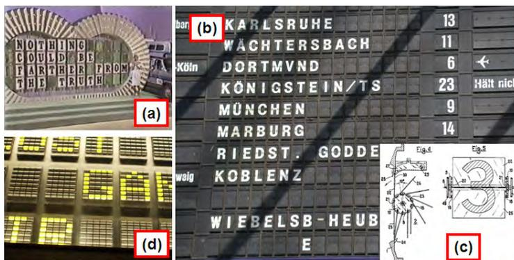
Figure 1.3: (a) an early “mechanical” display, (b) a picture of a split-flap display and (c) a drawing showing the principle, (d) a flip-dot display
