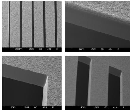
*Figure 2.9: Result of stencil fabrication: illustrating an excellent sidewall quality*
