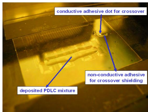
Figure 4.36: The PDLC mixture is deposited onto the bottom substrate after applying the crossover dot and an arc of shielding non-conductive adhesive
