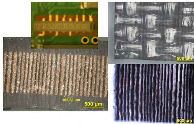
Figure 3.5: Zebra stripes: two top views (left), a side view showing the outer elastomeric material (top right), and a view explaining where the name “zebra stripes” originates from (bottom right, side view illuminated from the back)
