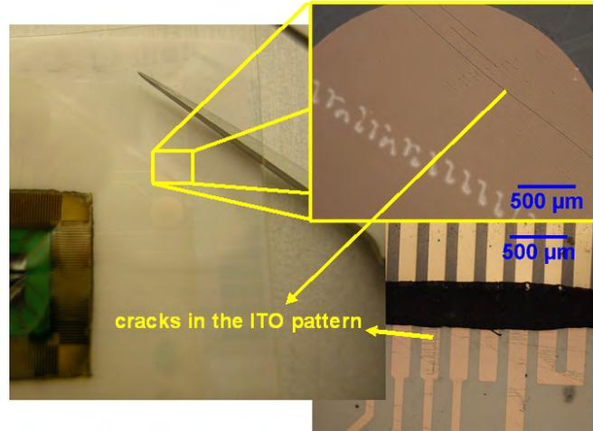
Figure 6.22: ITO cracking is a problem that can already occur during release of the PES substrate from the carrier
