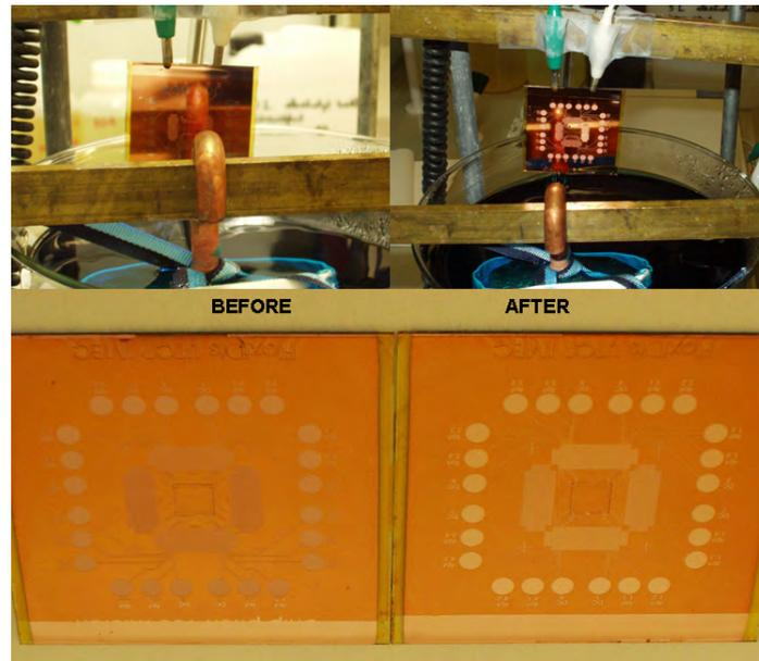
Figure 6.11: Electroplating the UTCP for the metallization layer by pattern plating
