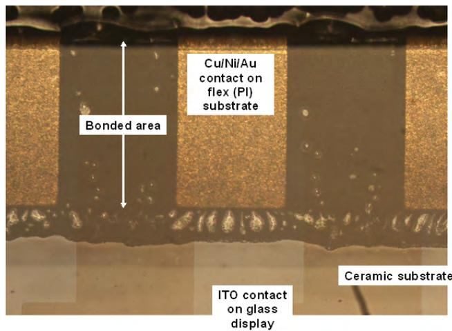
Figure 3.19: A close-up of the resulting display bonded to the flex substrate with ACF
