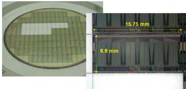
Figure 3.33: The row drivers used for the HeMind display
