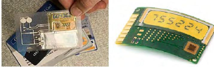
Figure 5.13: A prototype (left) and the Primero, a commercially available flexible display module for card applications (Aveso, Inc.); the used display technology is invented by The Dow Chemical Company and is based on electrochromism
